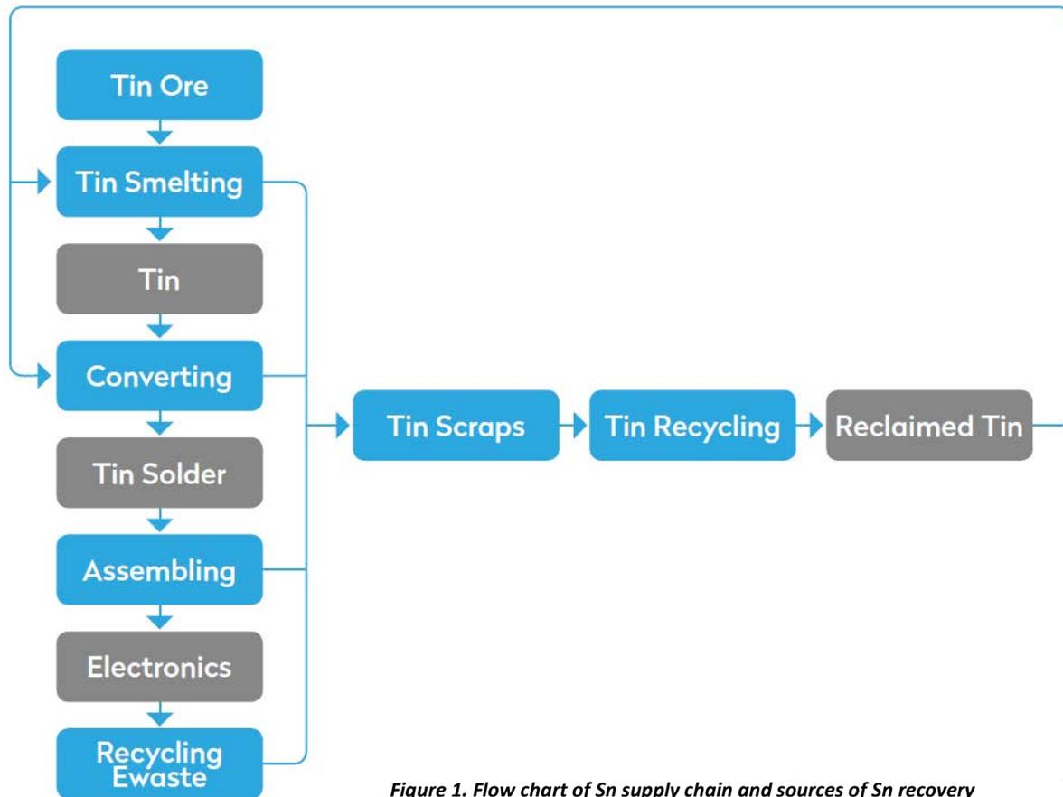
Figure 1. Flow chart of Sn supply chain and sources of Sn recovery
