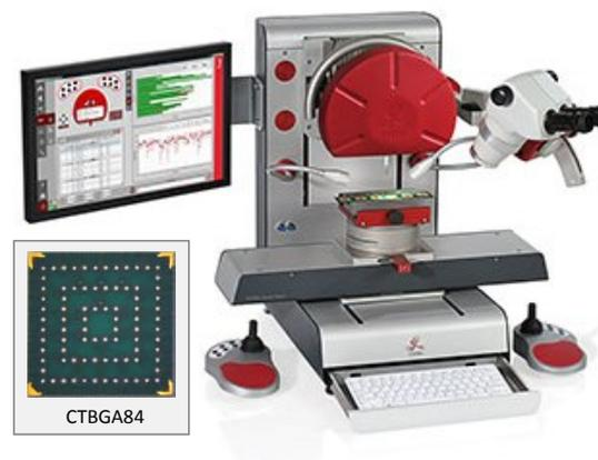
**Figure 1.** Condor Sigma bond tester. CTBGA84 (inset)
