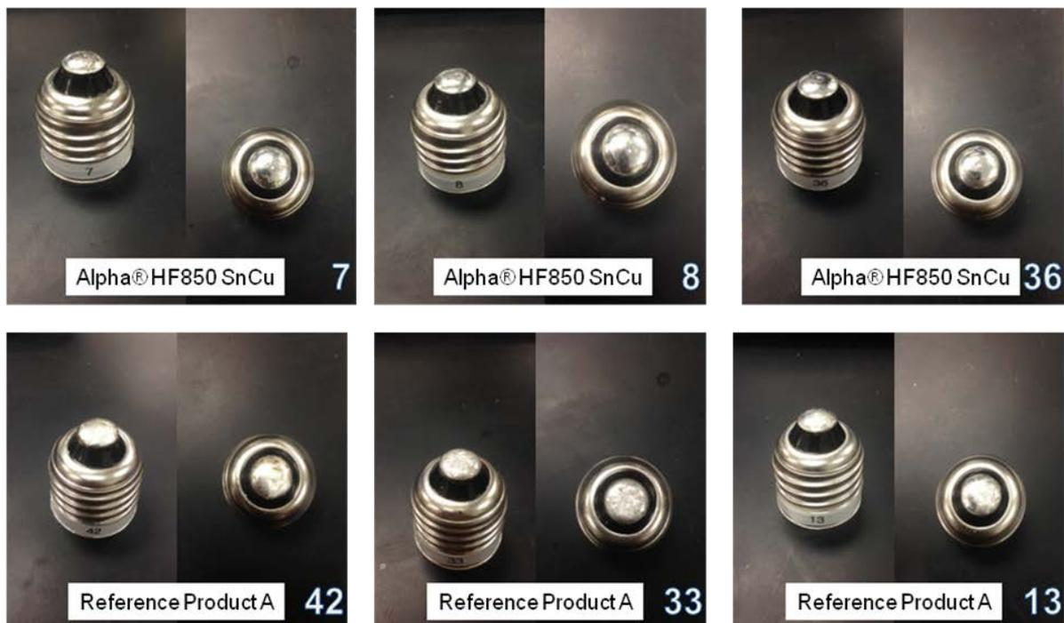
Figure 2. Images of randomly selected assembled end caps using reference cored wire and Alpha® HF850 SnCu
